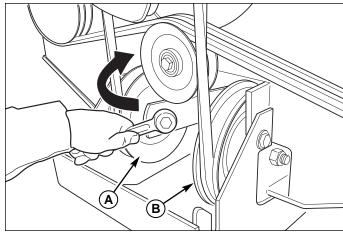
Figure 48. PTO Drive Belt Removal
